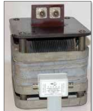
► Fig. 2: Vintage “Stop Coil” with the modern transformer version
