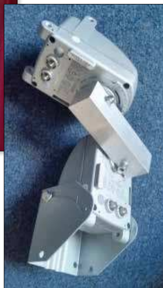
► Positioners connected by a custom joiner bar Photo and CNC milling: MODTS
