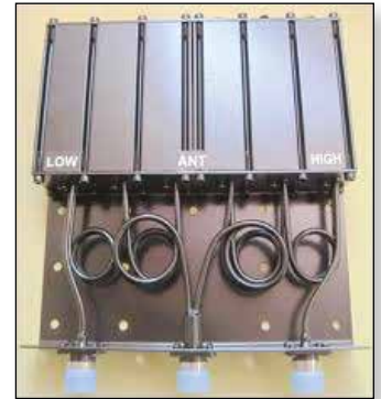
► A VHF diplexer similar to the one we used to provide a deep notch on the pager frequency of 153MHz. The central aerial socket is left open circuit and all cavities tuned in series.
