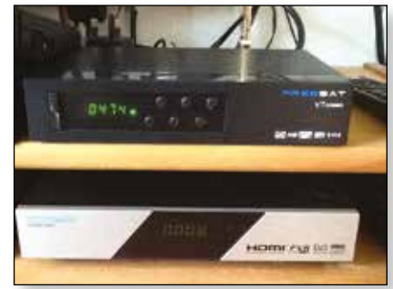
► Both of these satellite receivers will operate at 1ms/s with DVB-S2 & DVB-S. The Freesat v7 is currently available on Ebay for less than £30 and operates from 12V. The Icecrypt is an older model, but a very fine, sensitive receiver.
