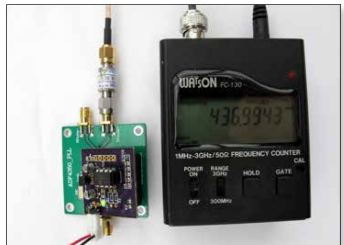
► Photo 3. The thin controller at work.
