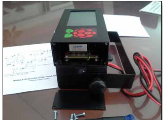
► The Nyquist filters are interchangeable through the side of the case
