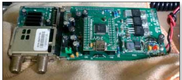
► A MiniTuner - see the BATC shop for details of the parts available to purchase.
