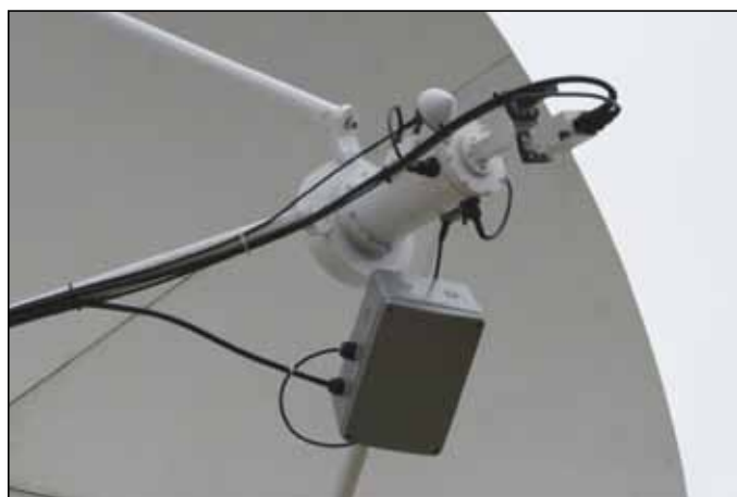
► S-Feed and preamplifier on the 3.8 mtr dish located at Goonhilly.
