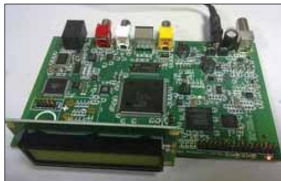
► BATC DTX I encoder, QPSK modulator and up converter
