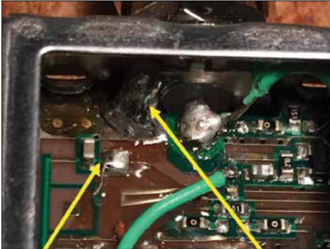
► Remove disconnected choke
