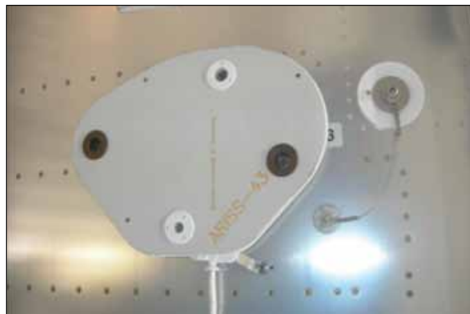
► One of the two patch antennas (ARISS-41 and ARISS-43) on the outside of the Columbus module.
