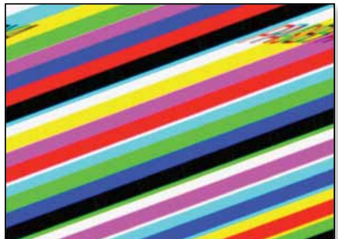
► With an incorrect sampling rate, the result is a slanted picture.
