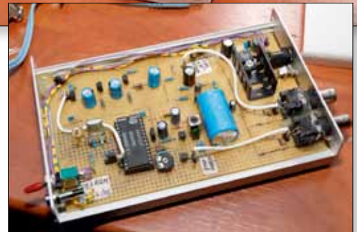
► Video sync generator built into a Euro Card Case
