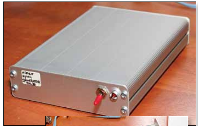
► Video sync generator built into a Euro Card Case
