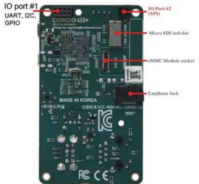
► Figure 5 – The bottom side of ODROID U3. The micro-SD memory slot is shown on right side near the top
