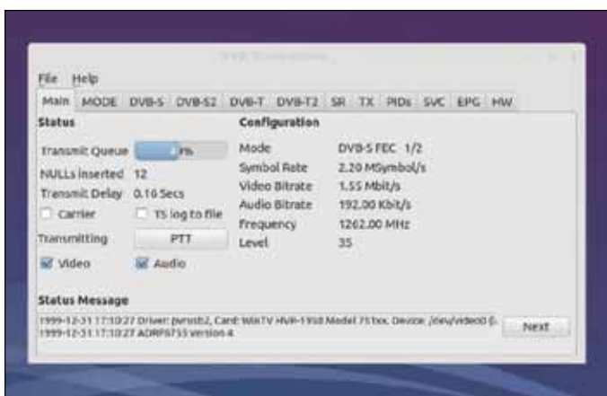
► Figure 7 – The DATV-Express GUI for ODROID looks essentially the same as when installed on Ubuntu on a PC
