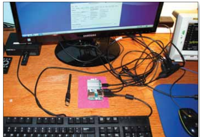
► Figure 8 – Set-up to use ODROID U3 to test with DATV-Express board at QTH of W6HHC
