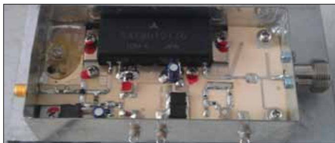
► Replacement 12 volt 23cm 20 watt PA, made by DGOVE from Germany, mounted on a heatsink
