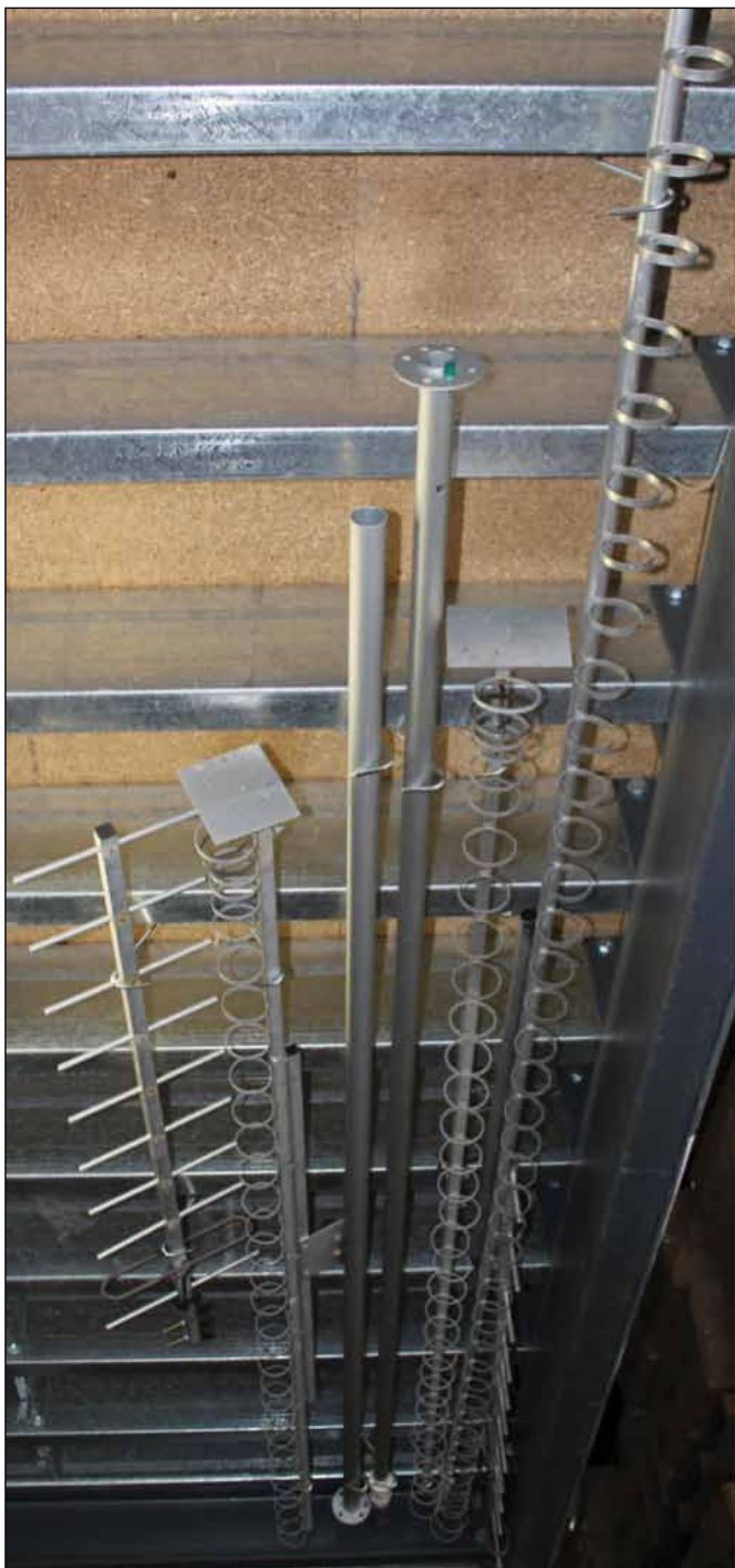
► Spare ATV 23cm TX & 70cm RX antennae and masts hanging from the roof
