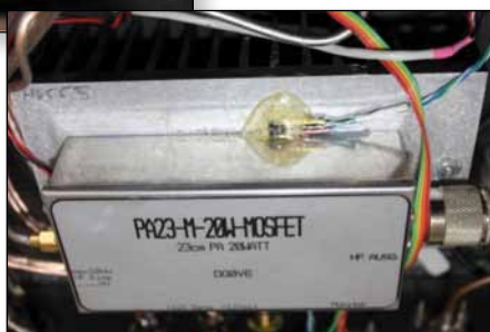
► Temperature sensor device in the glue
