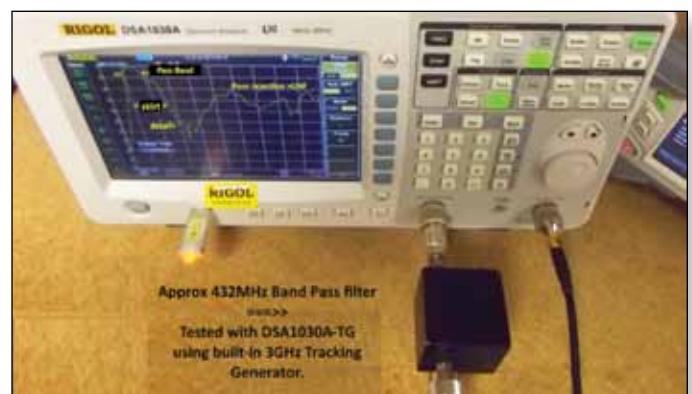
► Fig 5. Snap above isn't my best but does speak for itself; showing a black band pass filter under test.
