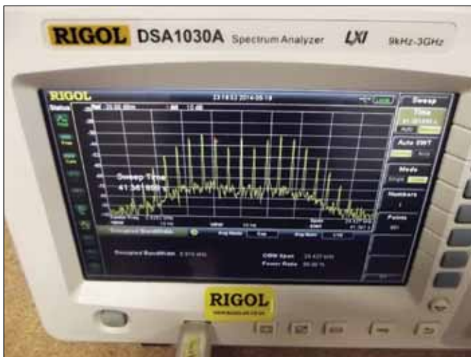
► Fig 4. - You can immediately see the carrier power now spread over a number of frequencies in the expected comb pattern for a phase modulated signal. As per theory the lines of this comb are 1.1 kHz apart (each of the ten horizontal squares is ~2.4kHz of the span).
