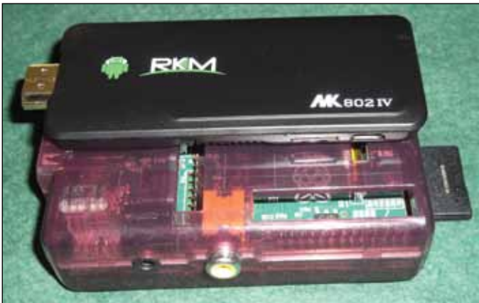
► An MK802 device sitting on top of a Raspberry Pi
