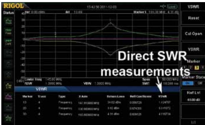
▷ The Rigol software DSA800-VSWR option measures values and displays SWR report
