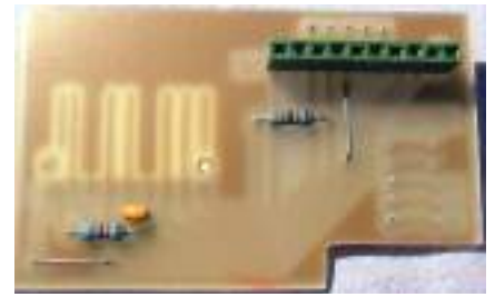
The interface board. Cutaway allows access to presets on main board.
