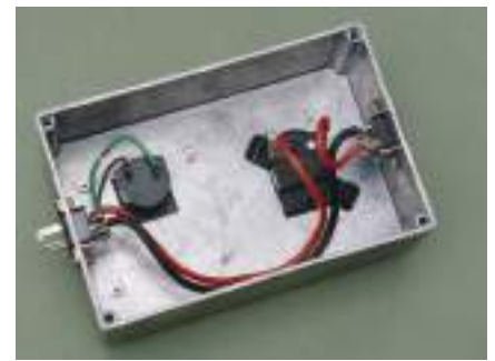
Fig. 6 Battery monitor - inside
