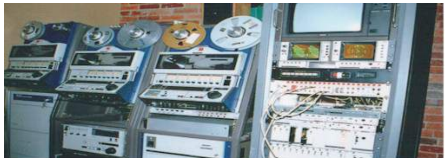
Three Sony C format VTR Machines, edit control rack, Beta SP deck distribution and monitoring
