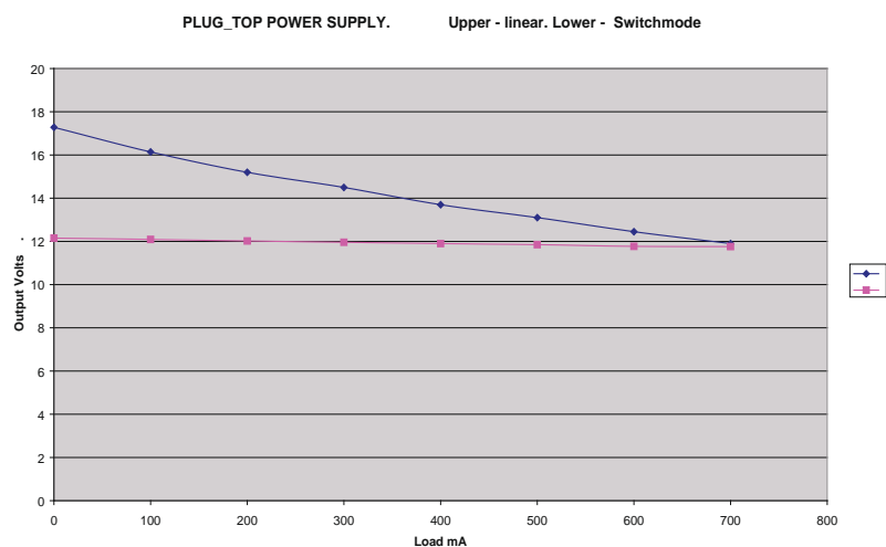
Fig.3. Graph showing output voltage v. Load
