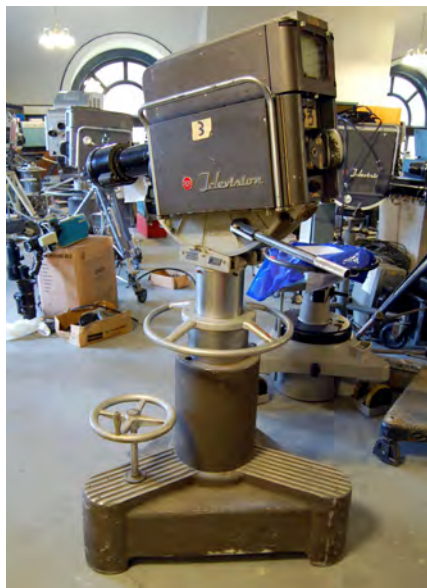
An RCA TK11A 3" inch image orthicon camera sitting on a PD1 pedestal. Very mechanical and very heavy
