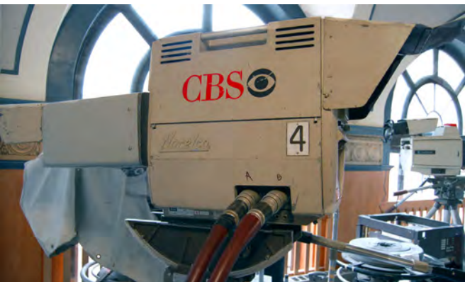
Dicky manhandles a TK41C. This 3-tube Image Orthicon camera type, (christened 'The Coffin' because it was wider at the rear than the front) was capable of producing, under the right conditions, very pleasant colour pictures.
