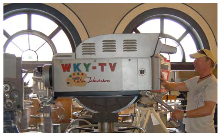
Dicky manhandles a TK41C. This 3-tube Image Orthicon camera type, (christened 'The Coffin' because it was wider at the rear than the front) was capable of producing, under the right conditions, very pleasant colour pictures.
