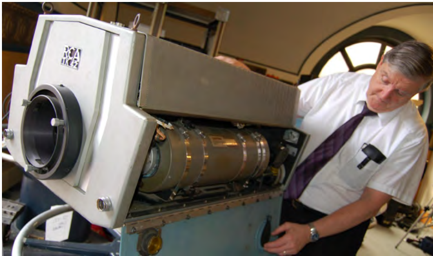
A TK 42 colour camera sans lens. Three 1" inch Vidicons and a 4 1/2" inch Image Orthicon tube combined. Not a happy mix. 'Muddy' flesh tones apparently
