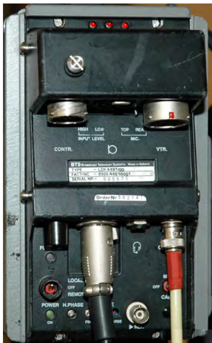
Rear of the EFP back with connectors for VTR and or CCU
