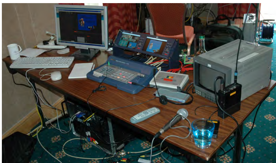
Our mobile studio, the new cues box just to the right of the vision mixer, and the new PC and rack case under the table
