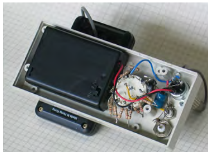
Fig.3. Internal view of the DTMF Tester
