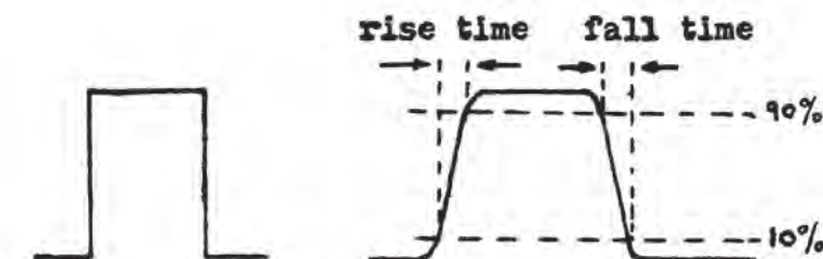
Fig.1: Ideal Pulse (L); practical reality (R).
