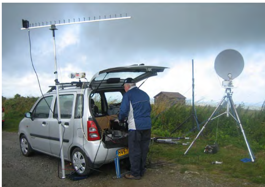
GW3PYB/P 23cm Masthead antenna and 60cm 10Ghz dish with storm clouds overhead.
