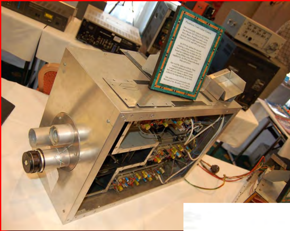
Home made 3-tube plumbicon
