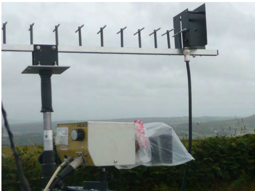
Low power ATV TX on 10.340Ghz feeding the GB3TM repeater just along the road at Nebo.
