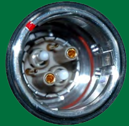
Close up of the near end, the fibres are the two white "pins"
