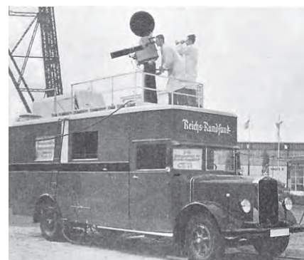
German Tv's 'Intermediate Film' OB Truck. Two of these 'delayed action' systems (could be at little as 15 seconds) used quick-processed film to cover selected events of the 1936 Berlin Olympic Games. Alas, no footage survives.
