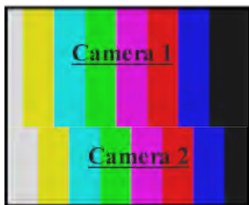
Camera 1 and 2 Need Line Phasing
