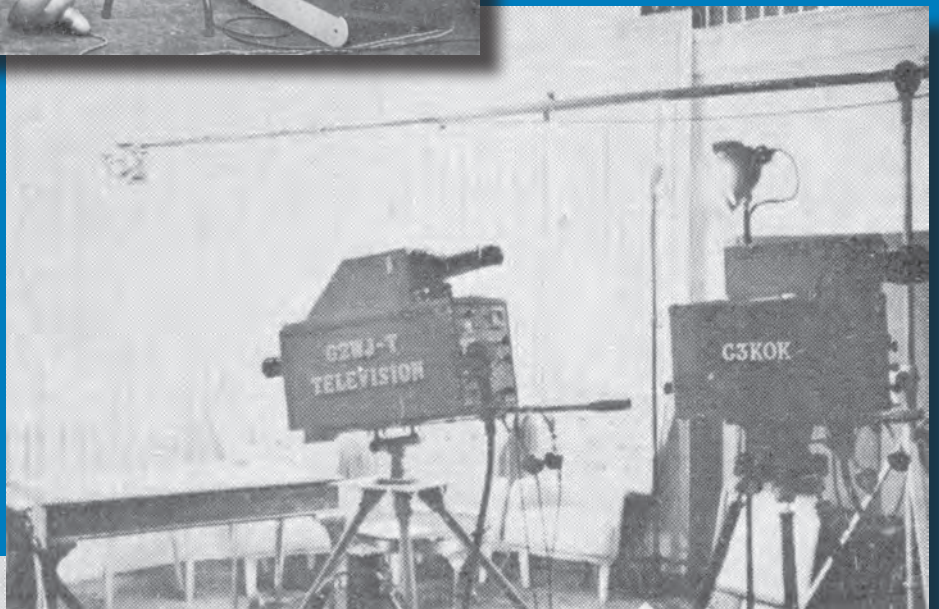
The Studio, showing the two cameras (photicon on the left, and image orthicon on the right) and mike boom, and what was described as 'comfortable seating'.
