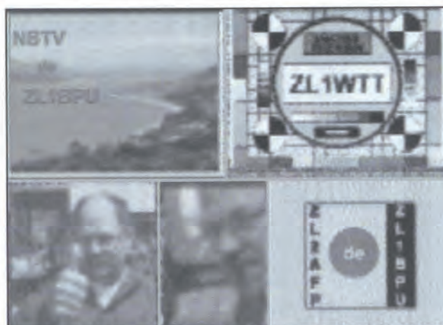
Figure 3. Pictures sent between Auckland and Wellington during the evening on 80 m, with frame rates from 3 fps (monochrome) to 0.2 fps (colour).
