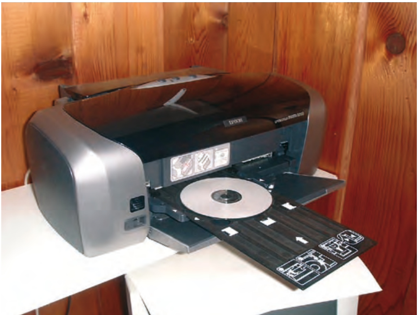
A printable DVD loaded in a special carrier prior to inkjet printing it's top surface.
