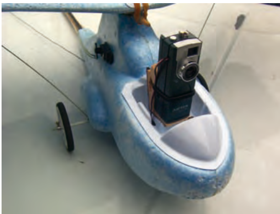
Aiptek camera mount showing external shutter control wire
