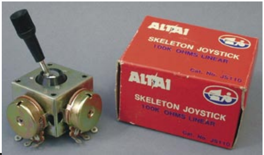
Figure 3 - Altai skeleton joystick
