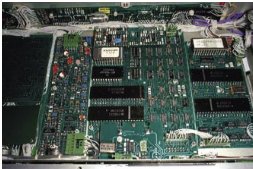
Audio 1 & 2 AGC Time code system Machine syscon CPU This view shows some of the circuitry mounted on the lower surface of the 'upper' electronics compartment, directly under the tape transport. There's a lot of hand wiring in this machine..
