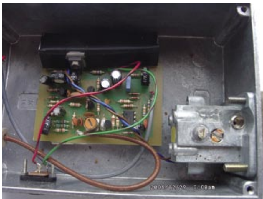
Bob Platts GunMod 2 pcb, feeding a Gunn diode Tx. picture by Graham Hankins G8EMX
