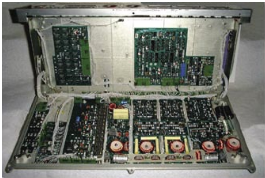
A view of the lower electronics compartment with the base plate un-screwed and lowered for access.
