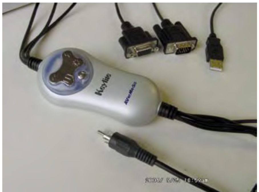
PC to TV converter. Unplug monitor from PC, and connect to VGA Out socket. Plug VGA In port on device to outlet on PC. Connect usb for power. Composite video produced at phono plug!
