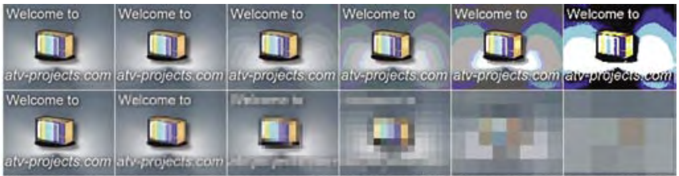
Fig 2 Top: L to R resolution halves each time, Bottom: L to R sampling halves each time
