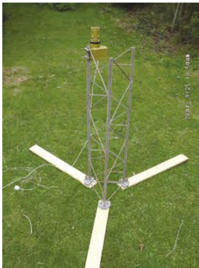
Portable Antenna support tower. 10ft lattice tower cut down to be manageable. Wooden extension 'legs' to ensure stability, attached by bolts and wingnuts for speed of assembly on site.
