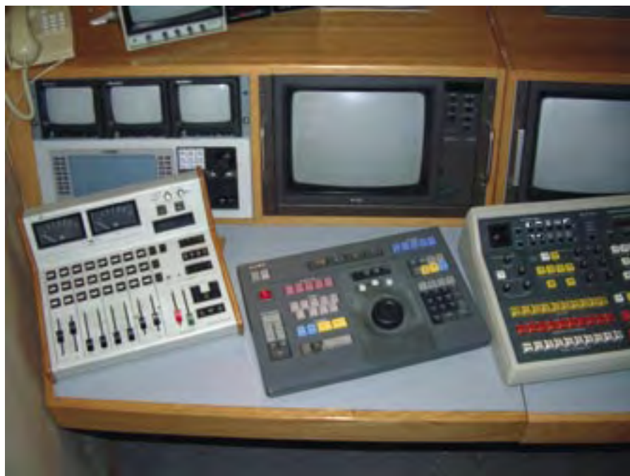
The final control desk. From left to right - Graham Pattern audio mixer, Sony BVE 2000 edit controller, and the GVG 100 vision mixer. The ADO is control panel is behind the Graham Pattern mixer
