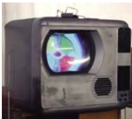
Figure 4 Gray Engineering CBS Monitor
