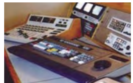
The MK2 control desk. Graham Pattern audio mixer Sony BVE 5000 edit controller
