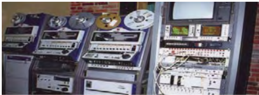
The business end, of the Mk2 edits suite Three Sony BVH 2000 machines. A BVW10 beta player and the BVE 5000 rack unit can be seen under the far left machine
