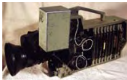
Figure 1 A Tired TK-76 Without Its Side Covers
