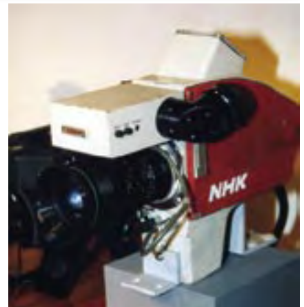
Figure 2A Ikegami NHK1 Camera Head
