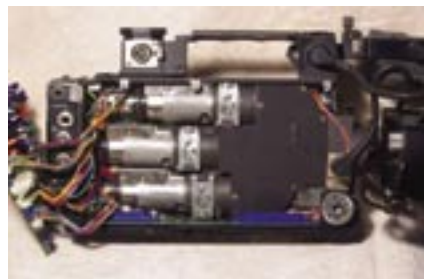
Figure 8 JVC KY-1900 Camera with Parallel Optics
