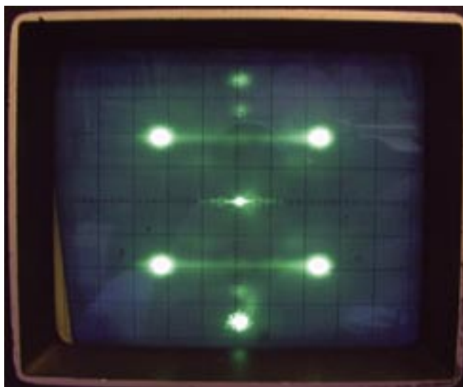
QPSK Modulation Constellation
