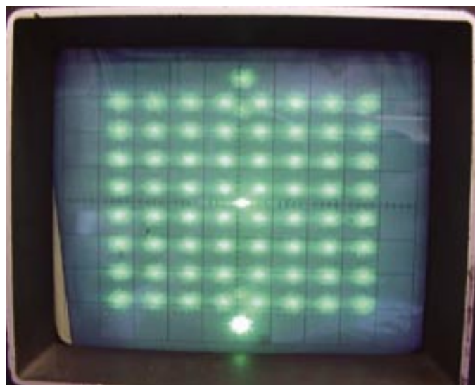
64QAM Modulation Constellation
