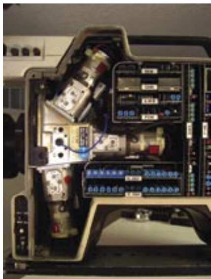
Figure 12A Ikegami ITC-730AP 3 Tube Prism Arrangement
