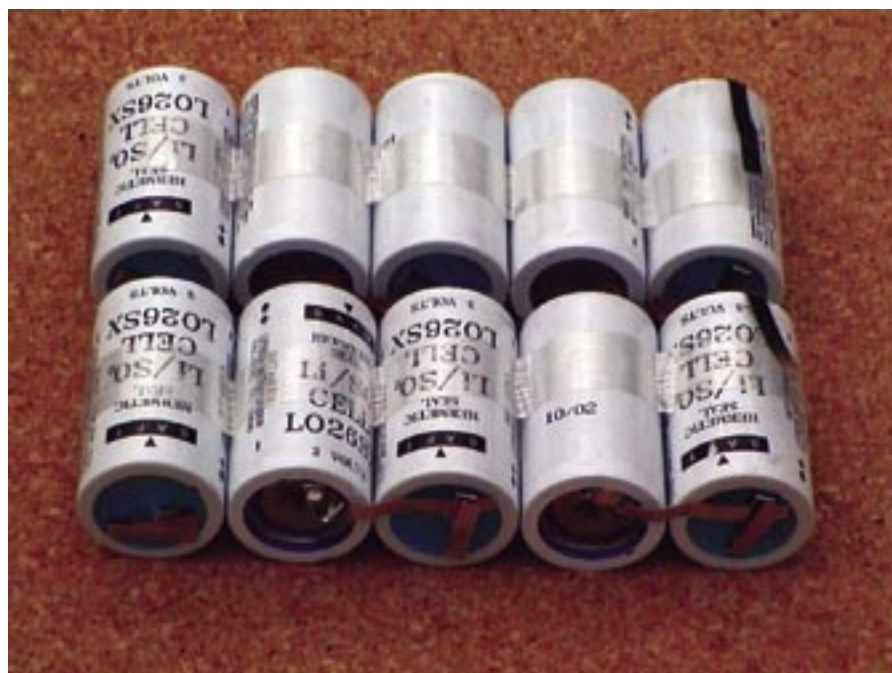
Figure 3 The lithium batteries
