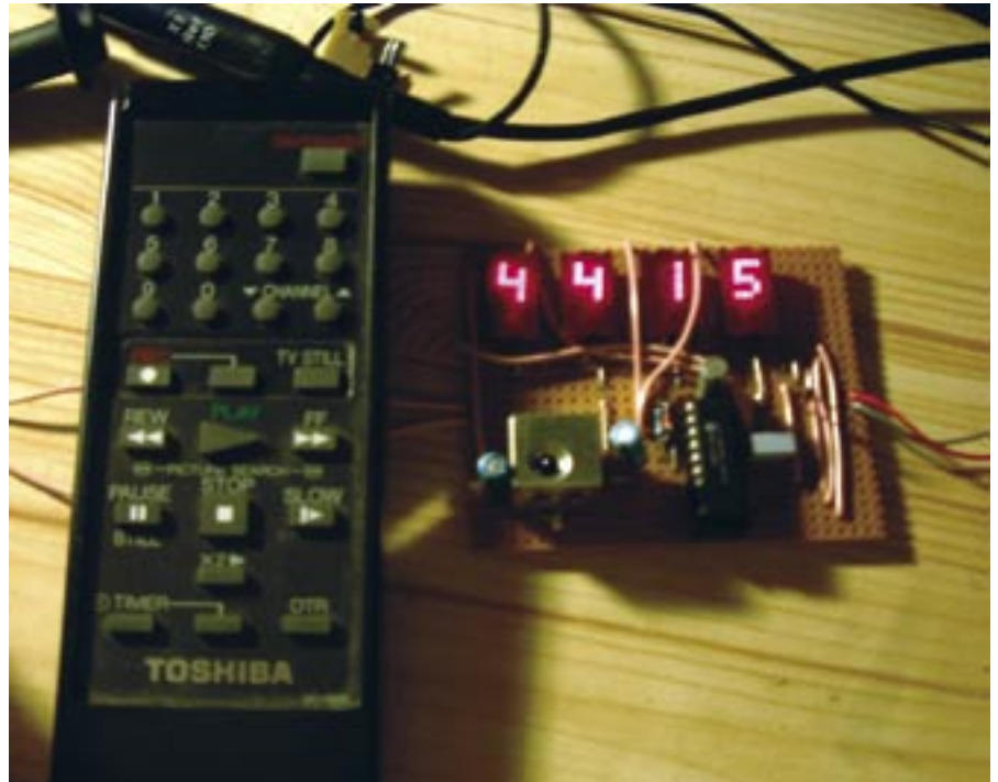
The Decoder showing GB3ZZ's video recorder address code of 44 and the PLAY command of 15. These were picked up by pressing the PLAY key on the remote control in the photograph
