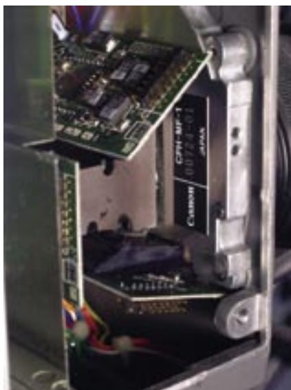
Figure 12B Ikegami HC-200 3 CCD Prism Arrangement.
