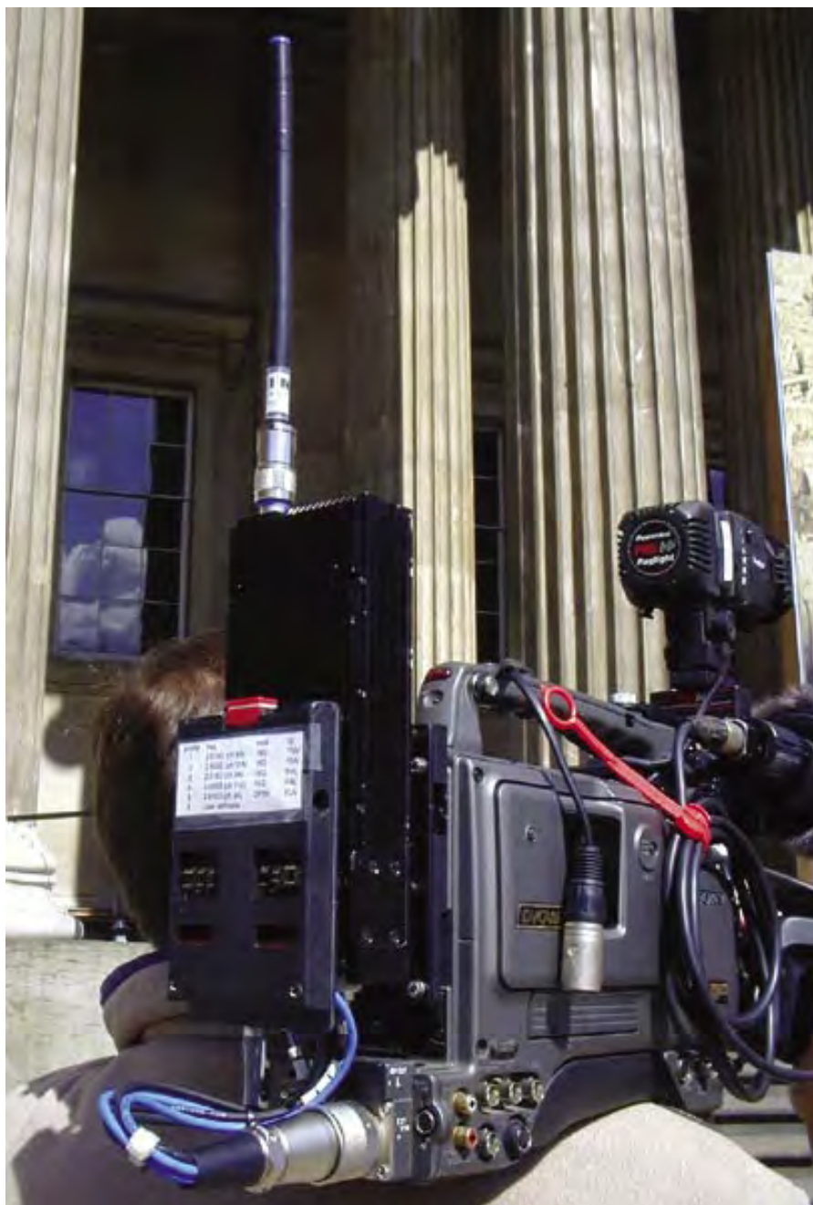
Broadcast MPEG COFDM transmitter (13cm)
