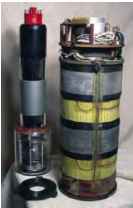
Figure 1 - 4-1/2 Inch Tube & Coils
