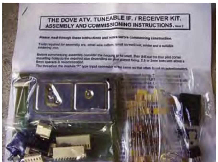
Dove 24cm receiver arrives by post with paperwork, components, tuner and PCB
