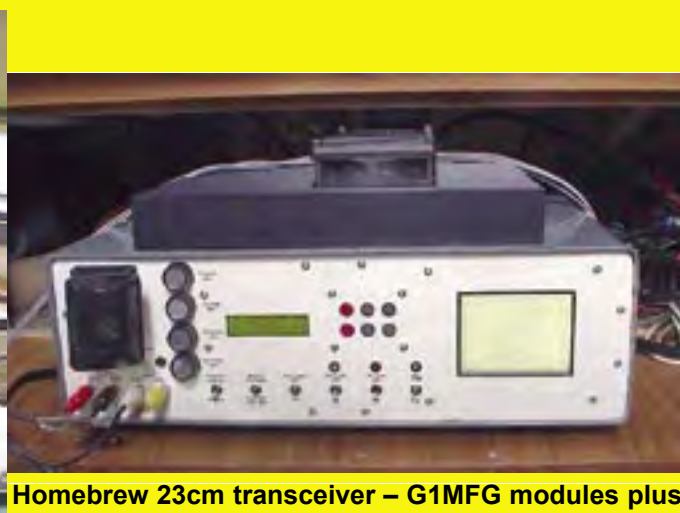
2m multimode rig, MM 70cm ATV Tx, MM 100W 70cm PA, 70cm 'brick wall' output filter, SSB Electronics 70cm preamp – all sitting on top of a 13.8V 40A linear PSU
