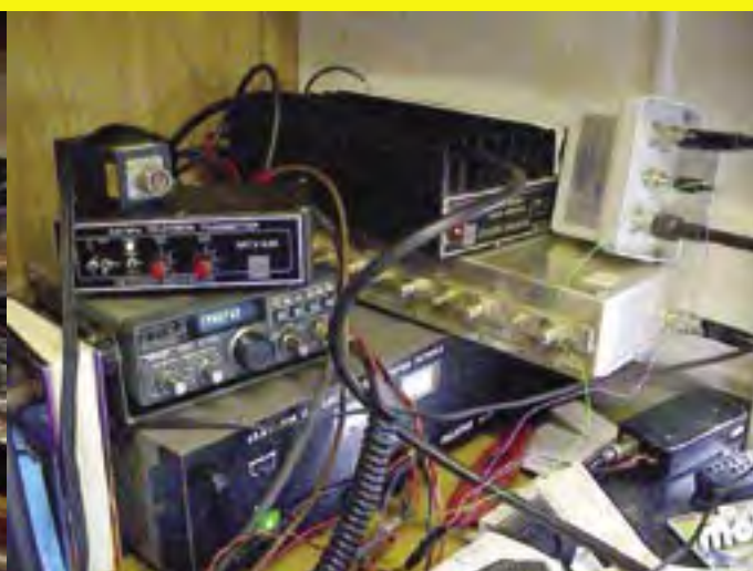
2m multimode rig, MM 70cm ATV Tx, MM 100W 70cm PA, 70cm 'brick wall' output filter, SSB Electronics 70cm preamp – all sitting on top of a 13.8V 40A linear PSU
