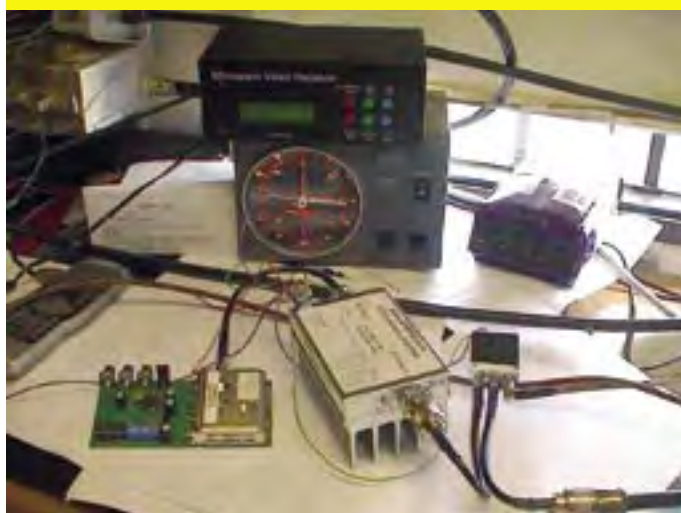
Rotator controller plus simple 13cm gear – G1MFG transmitter and 6W PA, co-ax relay, G1MFG Microwave Video Receiver
