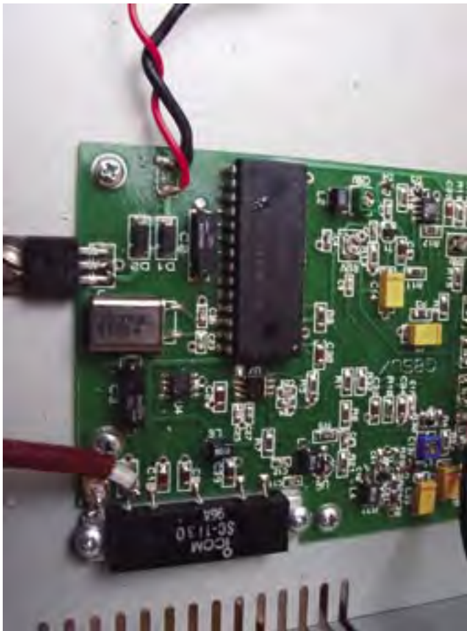
Suybuilt kit assembled - care needed with the surface mounted components and semiconductors
