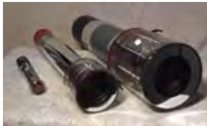
Figure 2 - 3 in. & 4-1/2 in. IO Tubes with a one inch Plumbicon Tube
