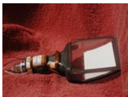
Photo 7 Sony FD CRT with Yoke
