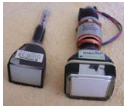
Photo 16 CRTs (L) BW: 40CB4 Colour: A04JGM09X with yoke
