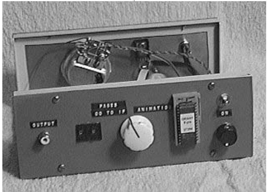
Front panel of the prototype unit. The socket on the PCB is connected to a ZIF socket on the panel by means of ribbon cable
