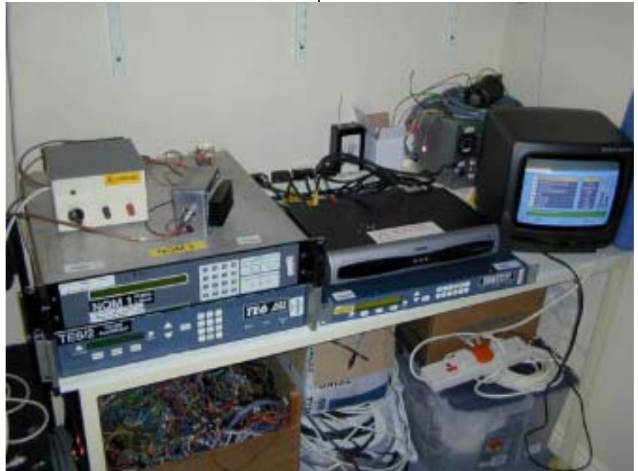
DATV equipment testing back to back, left bottom MPEG Coder, left top Modulator, right bottom professional RX and right top Nokia 9650S domestic receiver
