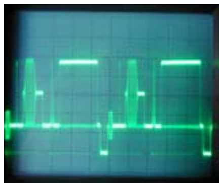
Received pulse and bar test signal on a scope (line rate)
