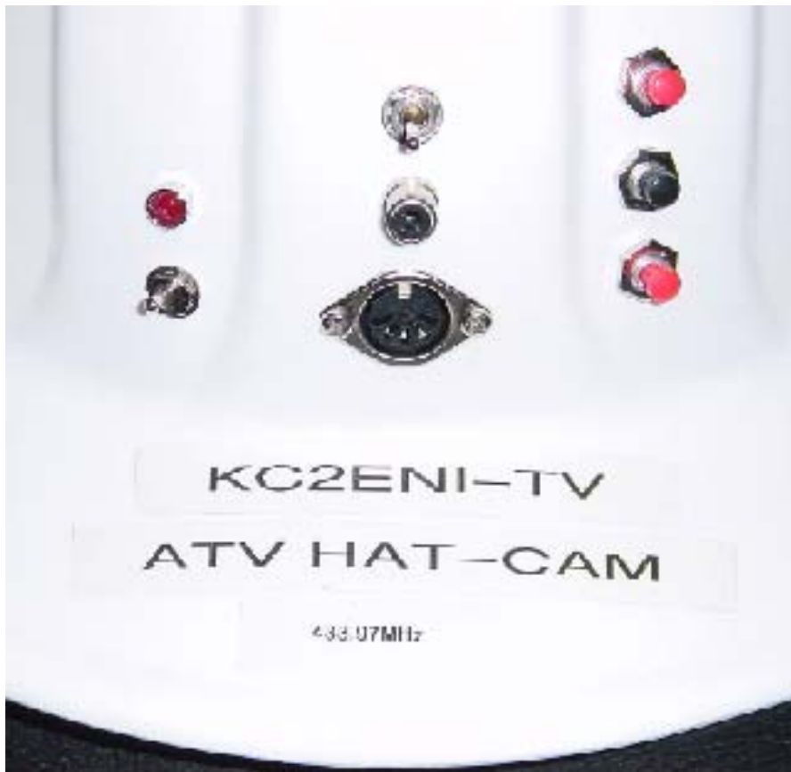
The power switch with its light
