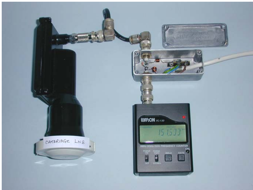
Figure 4 – 10GHz frequency measurement
