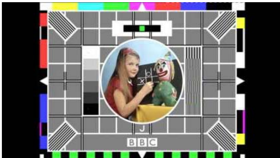
4:3 picture in a 16:9 coded frame
