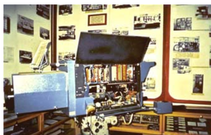
KT-116 4 tube colour TV camera, 1968 (side covers open).
