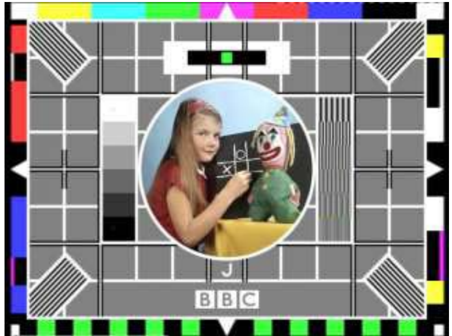
4:3 picture in a 4:3 coded frame
