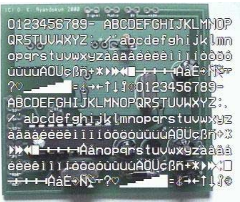
The output of the demonstration program. The STV5730A character set consists of 128 text and graphics characters that can be displayed on screen in a 28 column by 11 row grid.
