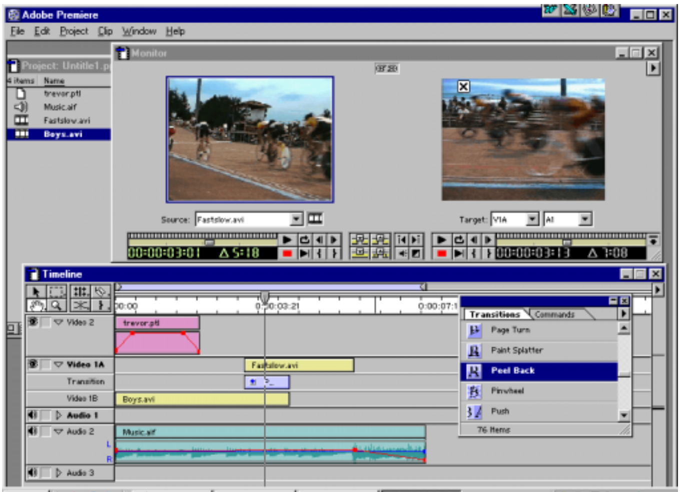
Figure 1 shows a caption set to fade in and out, two video clips with a transition and a sound track with fade out. The mauve bar sets the preview and the scrub pointer can be seen along with Transitions menu PV and TX monitors.
