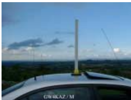
Picture 4 - Shows the Alford Slot antenna fixed to the mag-mount on the roof of the car, with the view toward GB3TM on the horizon over Anglesey, to the northwest.
