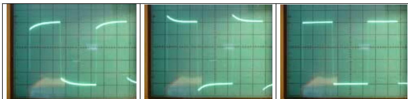
Fig.2. 'Scope traces showing Under, Over, and Correct (level) of probe compensation
