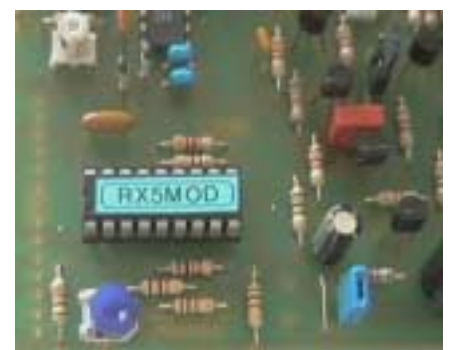
The heart of the receiver; the pre-programmed PIC chip
