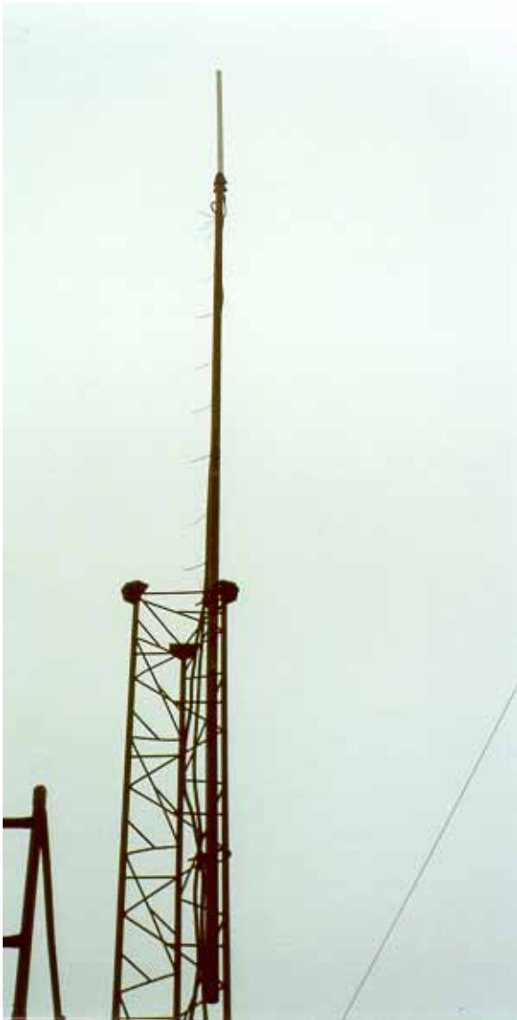
Two views of the dual Alford slot antenna used by the Beacons repeater groups' 1.3GHz ATV repeater. See 'TV on the Air' for more details.
