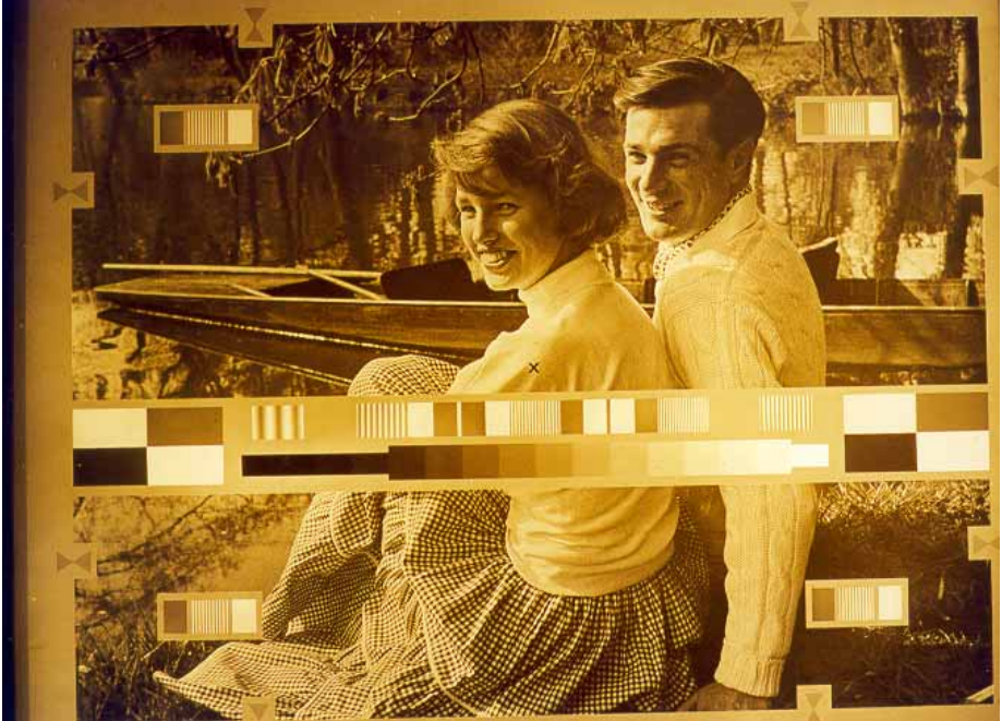
Light box slide used for the Iconoscope test
