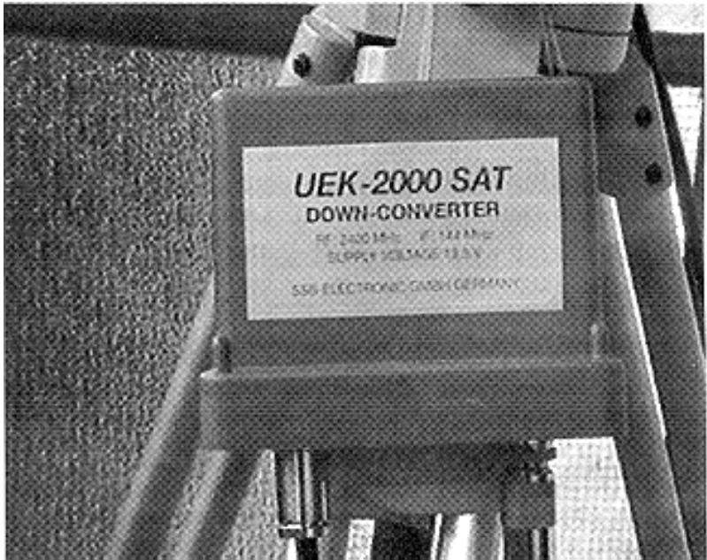
Figure 6. The downconverter used for these trials was the UEK-2000 from SSB Electronic (available in the UK from Piper Communications, Berks.).
