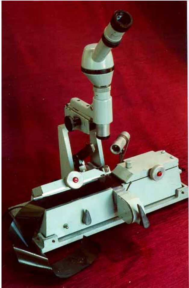
VT tape editing the easy way! Just find the pulses with a microscope and cut with a sharp object. This is the Smith's 'Micro 40' hi-tech VT editing machine from the 1960's
