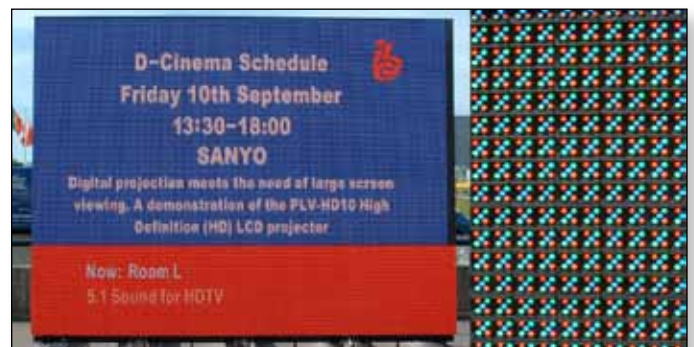
▷ LED Display with close up of pixels c. 2004
