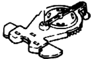
The pendulum drive assembly of the SL-C20, which seizes up.
