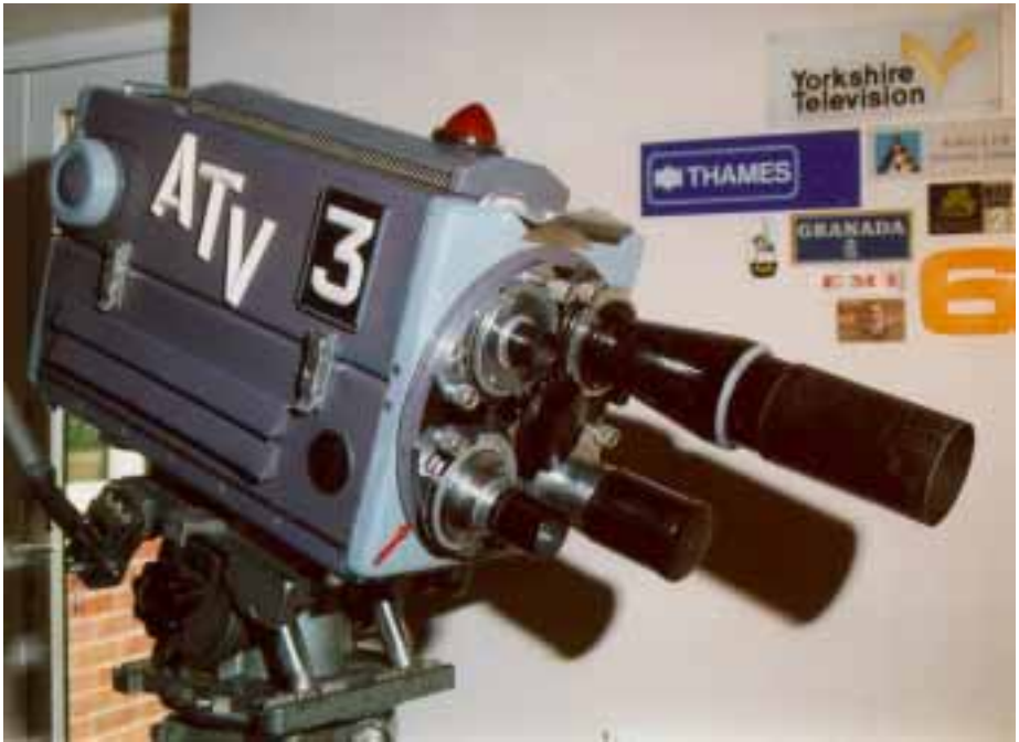
The Pye MkIII 3 inch image orthicon camera. (1956)
